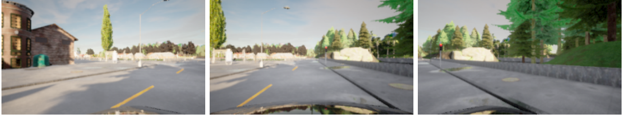
Fig. 1. Images from the three frontal cameras located at the left, central, and right part of the vehicle, respectively. They were taken after the first few interactions of the agent in the CARLA simulation environment considering our defined trajectory. Each camera produces a RGB image with 144 pixels of height and 256 pixels of width. These images are fed to the networks as they are.
